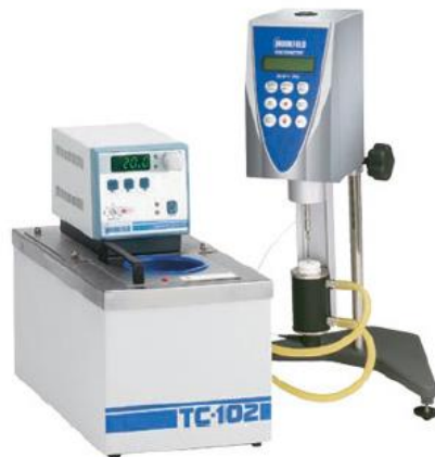
Fig. 1. the Brookfield Viscometer and its connection to thermo bath.
