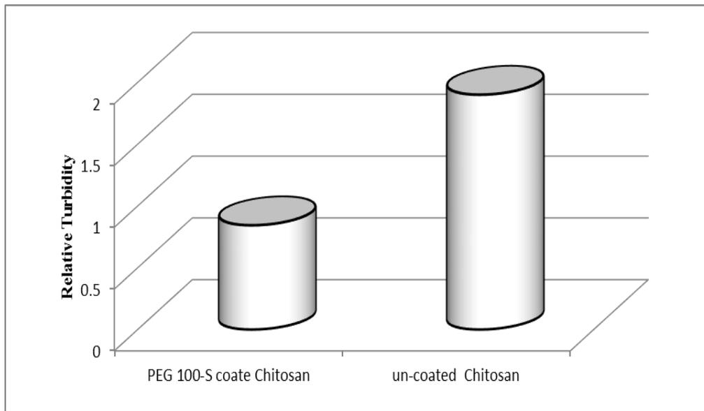
Fig. 3. Relative turbidity (Relative turbidity is the ratio between the absorbance [Optical density (OD)] at  $\lambda = 225$  nm after 1 h and before incubation)
