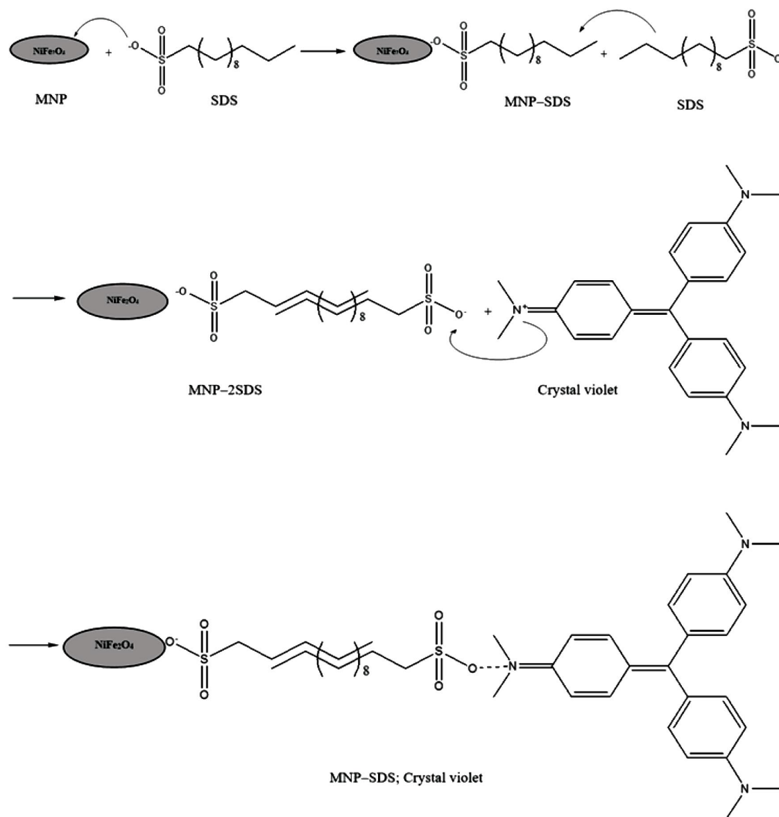
Fig. 5. The scheme is illustrating the modification process used to coat NiFe 2 O 4 MNPs with SDS and suggested mechanism of adsorption of crystal violet onto NiFe 2 O 4 -SDS MNPs.
