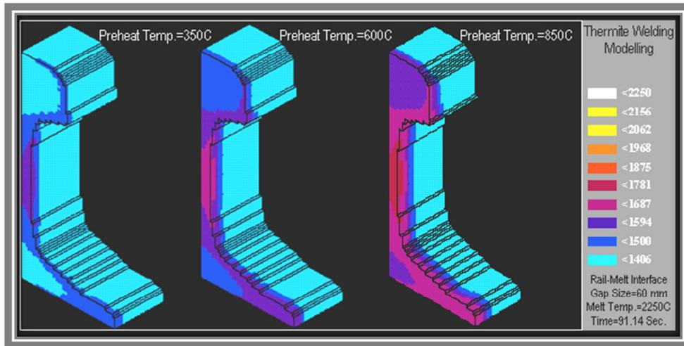
Fig. 9. Effect of preheating temperature on melt penetration
