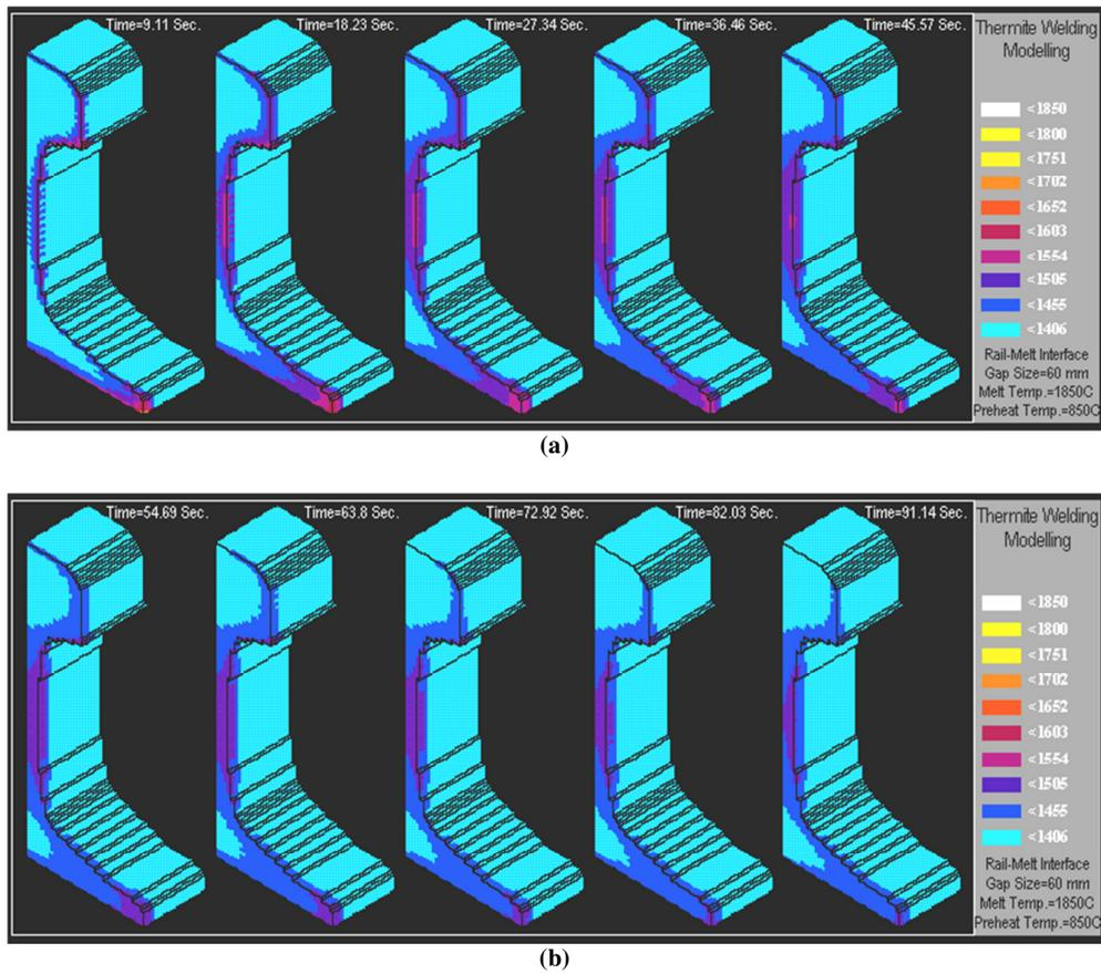
Fig. 6. Isothermal profile at  $S_1$  condition: (a) Time 9.11 sec.-45.57 sec (b) Time: 54.69sec.-91.14 sec.
