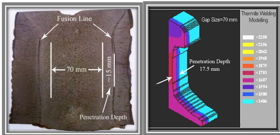
Fig. 5. Comparison between amounts of melt penetration obtained from the experimental measurement with the simulation result at  $S_5$  condition.
