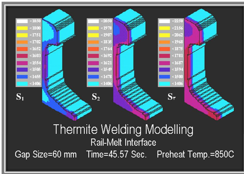
Fig. 7. Effect of initial melt temperature on melt penetration.
