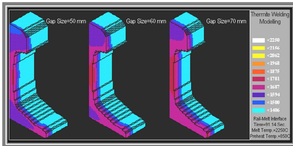
Fig. 8. Effect of gap size on melt penetration.
