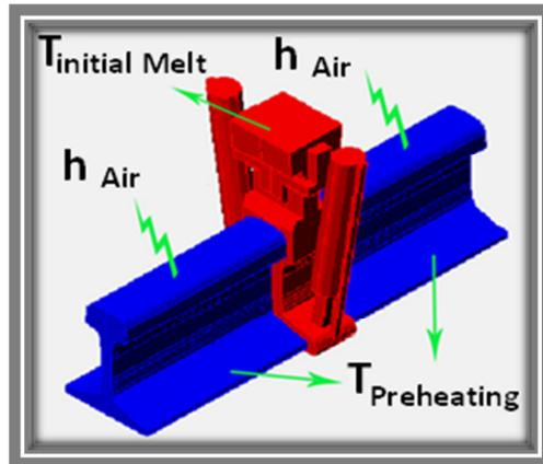
Fig. 3.Initial and boundary condition.
