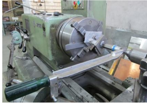
Fig. 5. The location of tools before the starting of the twisting process.
