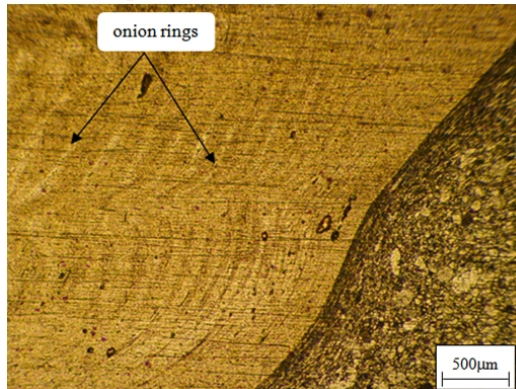
Fig 6. Onion rings in the stir zone.
