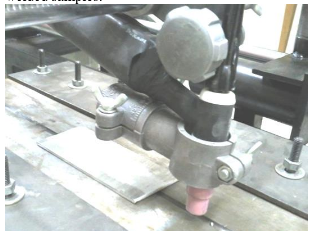
Fig. 3. Automatic TIG welding machine
