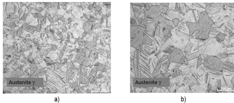
Fig. 1. a) Microstructure of 316L stainless steel at 50X and b) at 100x
