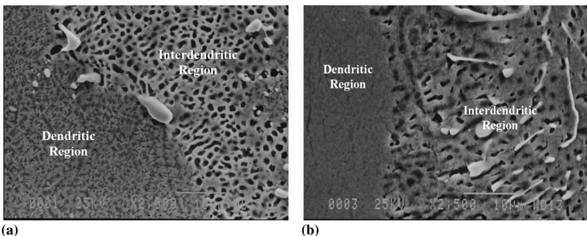
Fig. 5. SEM micrographs of the serviced superalloy after solution treatment at (a) 1295°C for 3h, (b) 1330°C for 3h.
