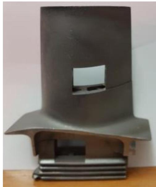
Fig. 1. Ex-service turbine blade.
