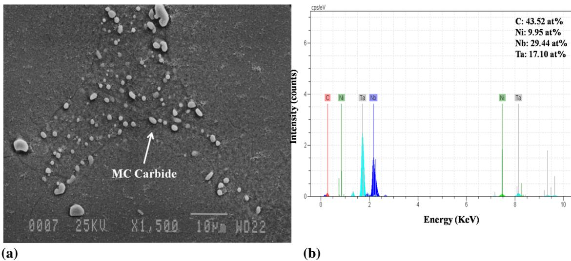
Fig. 6. (a) SEM micrograph and (b) EDS spectra taken from MC carbides after solution treatment at 1350°C for 3h.
