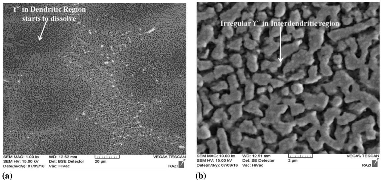
Fig. 4. SEM micrographs of the serviced superalloy after solution treatment at 1285°C for 3h.
