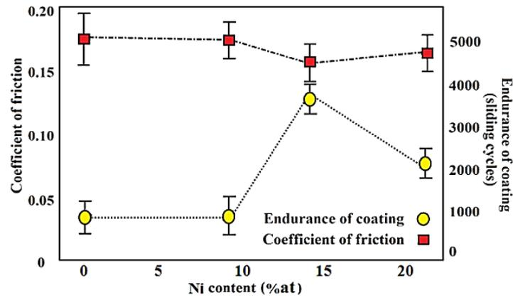
Fig. 10. Average friction coefficient and endurance of coatings test results of MoS<sub>2</sub>/Ni composite coatings with different Ni contents.
