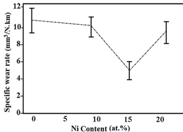
Fig. 11. Wear rate of MoS<sub>x</sub>/Ni composite coatings as a function of Ni content.
