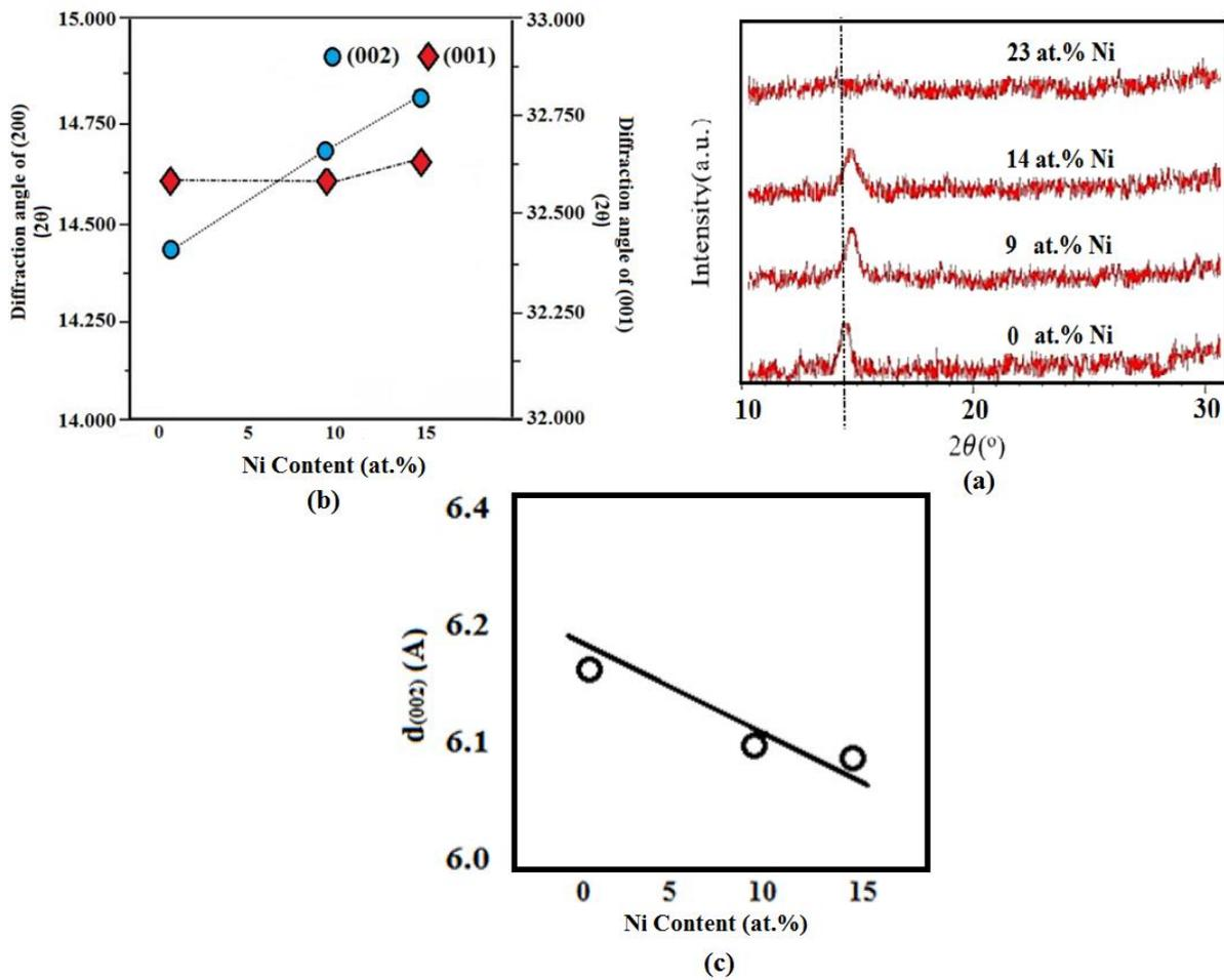
Fig. 4. Analysis of Ni doped MoS<sub>x</sub> coatings by XRD. (a) Diffraction angle of MoS<sub>2</sub> coatings containing varying amounts of nickel deposited at at the diffraction angle of about 14.5°, (b) The diffraction angle value of 2θ for the (002) plane vs. nickel dopant, (c) Changes in d-spacing for the (002) plane vs. nickel dopant.
