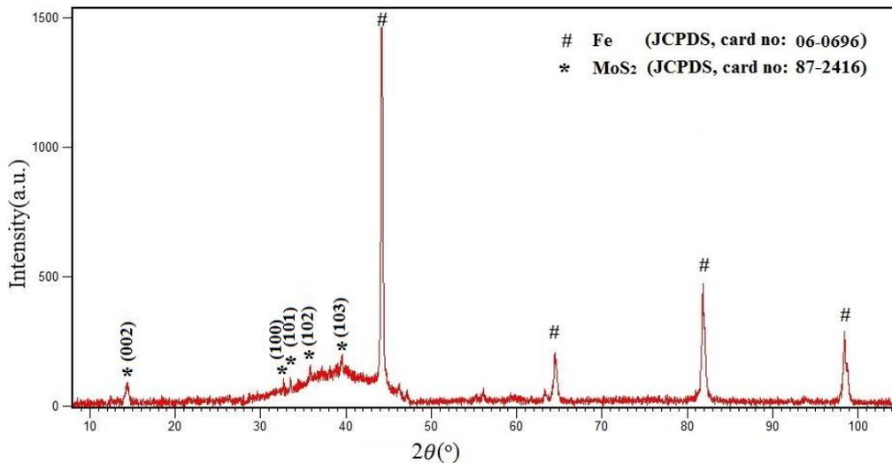
**Fig. 2.** XRD pattern of MoS<sub>2</sub> coating.
