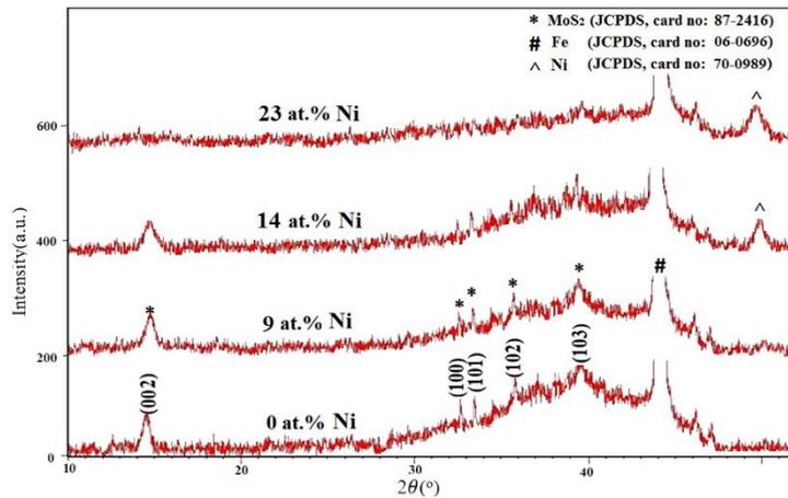
Fig. 3. XRD patterns of MoS<sub>2</sub>/Ni composite coatings with different Ni content.
