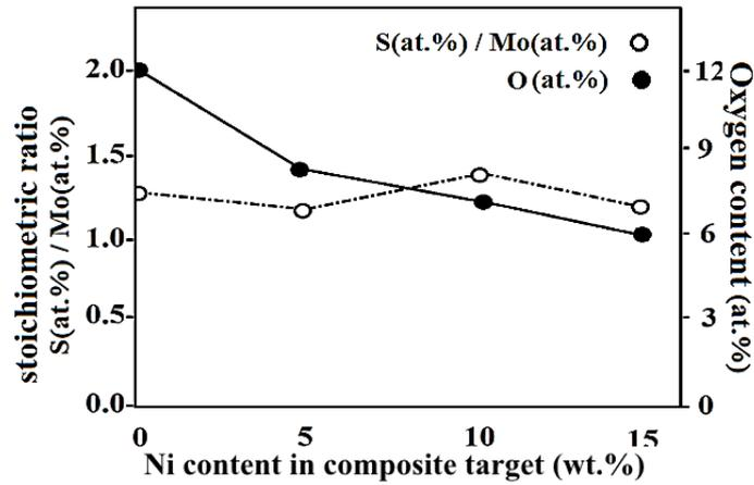
**Fig. 1.** The stoichiometric ratio and Oxygen content of MoS<sub>x</sub>/Ni composite coatings with different Ni content in composite target.
