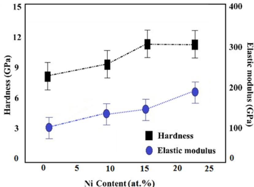
Fig. 5. The hardness and elastic modulus results of the  $\text{MoS}_x/\text{Ni}$  composite coatings as a function of Ni content.
