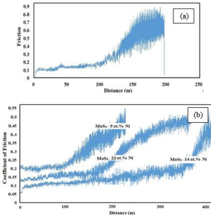
**Fig. 9.** Variation of the friction coefficient as a function of wear distances for (a) Pure MoS<sub>x</sub> and (b) MoS<sub>x</sub>/Ni composite coatings during the pin-on-disc wear test.
