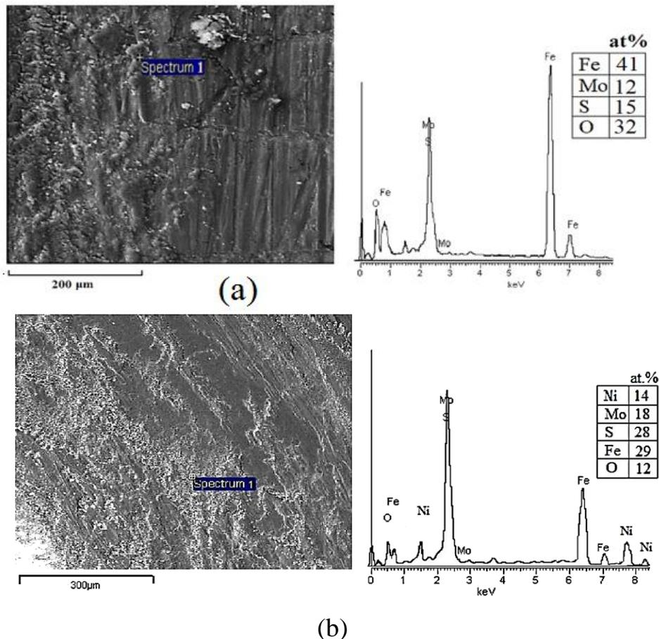
Fig. 12. Worn morphologies and EDX analysis of the (a) pure  $\text{MoS}_x$  (b)  $\text{MoS}_2/\text{Ni}$ , 14 at.% Ni after 800 wear cycles.
