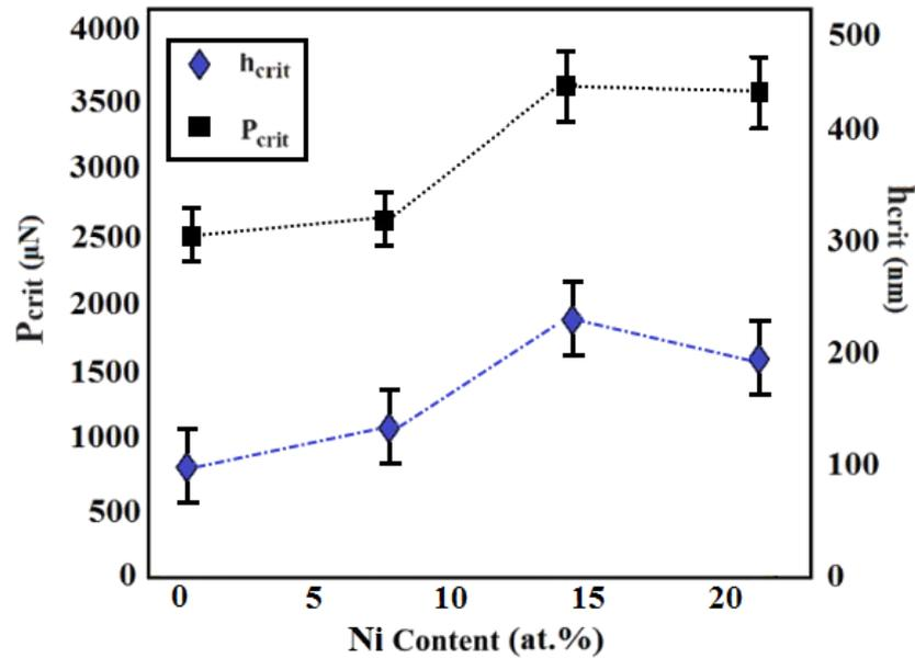
Fig. 6. the  $P_{crit}$  and  $h_{crit}$  results of the  $\text{MoS}_x/\text{Ni}$  composite coatings as a function of Ni content.
