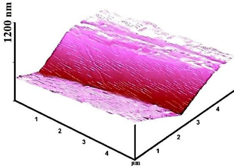
Fig. 7. 3-D in-situ SPM image of  $\text{MoS}_x$  coating after a 4000  $\mu\text{N}$  ramping force nanoscratch test.
