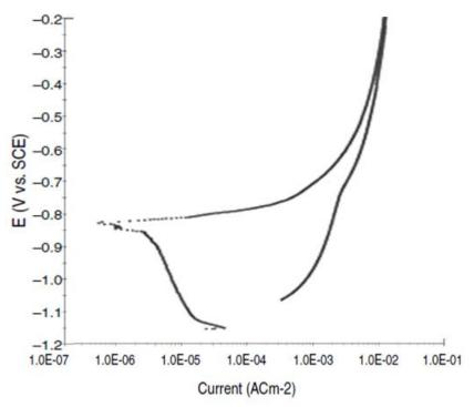
Fig. 6. Cyclic polarization graph of Al6061-T6.
