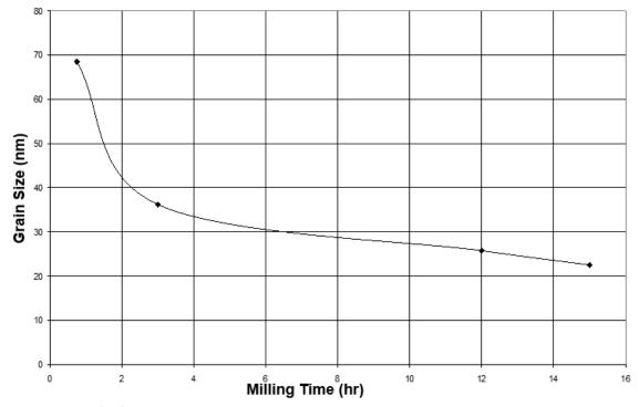
Fig. 3. Changes rate of Al6061 alloy grains size per milling time after annealing.
