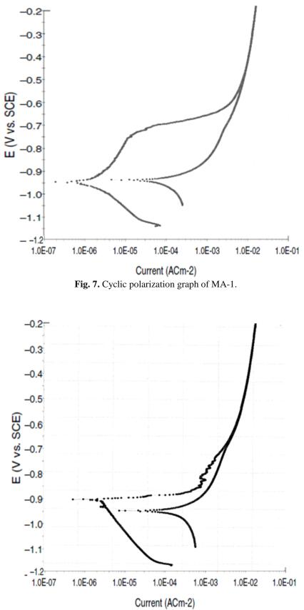
Fig. 8. Cyclic polarization graph of MA-A16061 / 1.25 TiB<sub>2</sub>.
