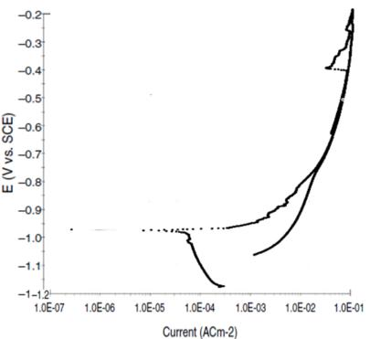
Fig. 9. Cyclic polarization graph of MA-Al-6061 / 2.25TiB<sub>2</sub>.
