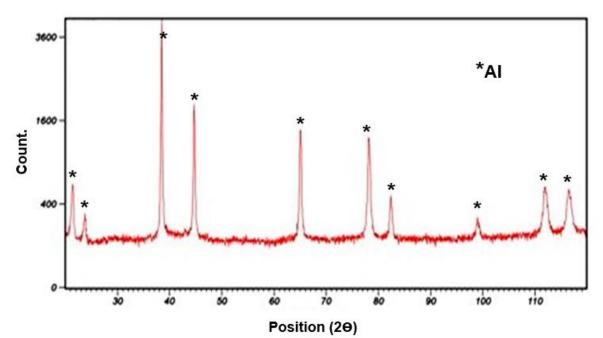
Fig. 4. XRD test results on the extruded MA-Al-6061 / 1.25TiB<sub>2</sub> composite alloy.
