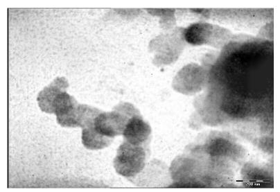
Fig. 1. The size of Al6061 powdered particles after 15 hours of milling by using TEM.
