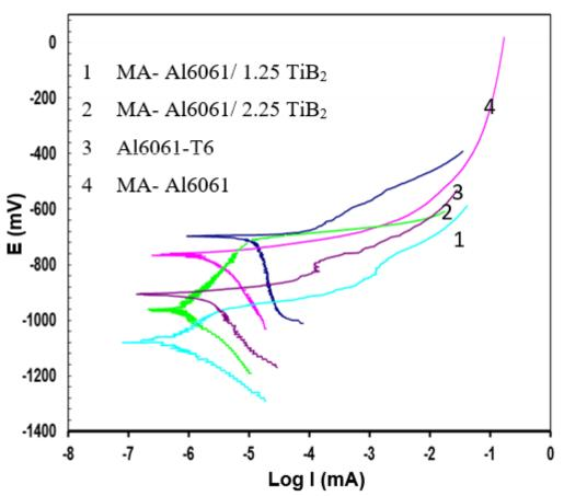
Fig. 5. Polarization test graphs of extruded nanocomposite samples.
