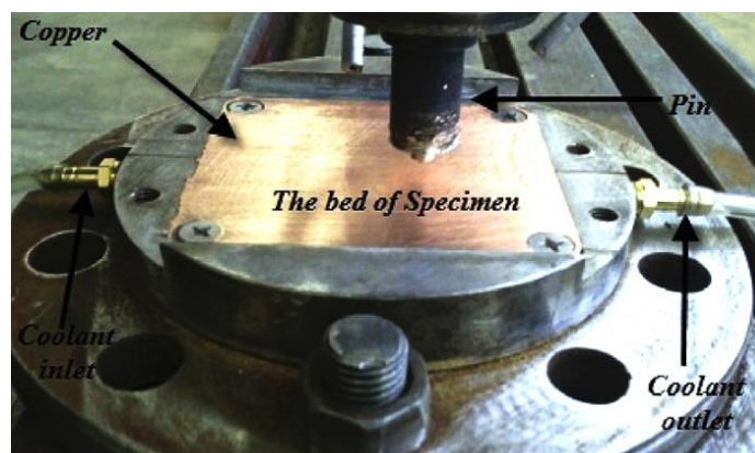
Fig. 1. The die used for cooling in the FSP.
