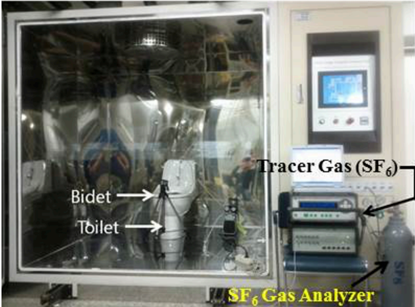
Figure 6: Toilet bowl-bidet system in environmental chamber
