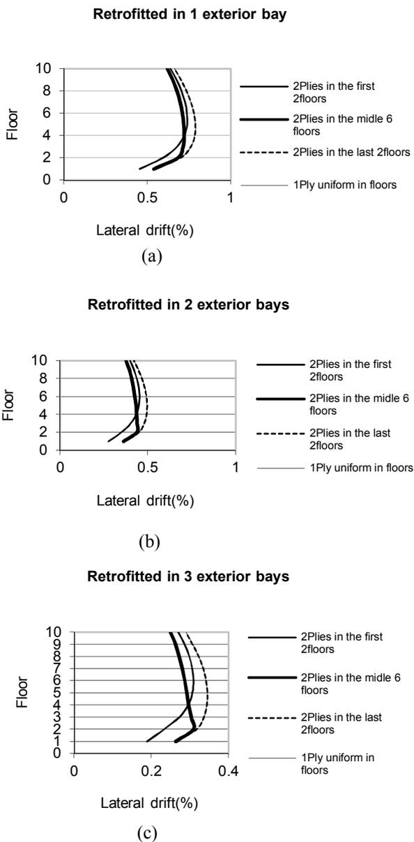
Figure 16. Variation of FRP ply at elevation with different bays
