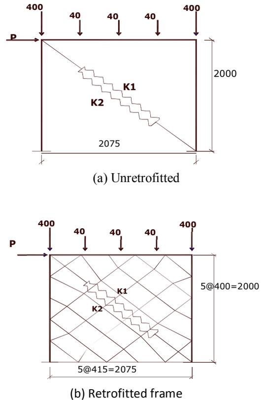
Figure 8. FE model for unretrofitted and retrofitted frame
