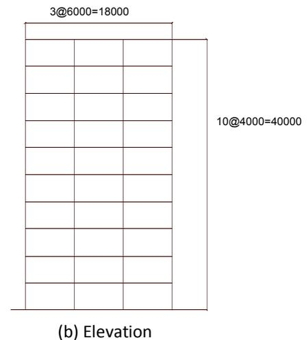
Figure 12. 10-story building subjected to retrofit system (All dimension, mm)
