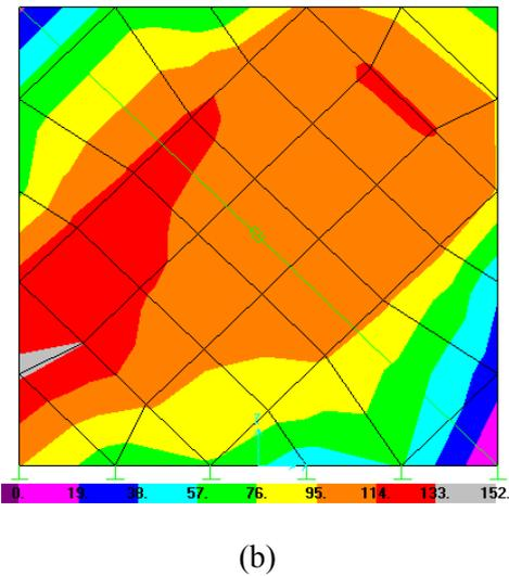
Figure 11. (a). Lateral load-Stress curve in central shell element, (b) Maximum stress distribution in FRP shell element
