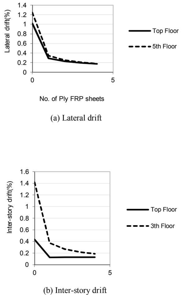
Figure 15. Effect of FRP thickness on drift (Uniform retrofitted at 3bays)
