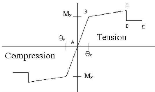
Figure 6. Flexural behavior of frame element
