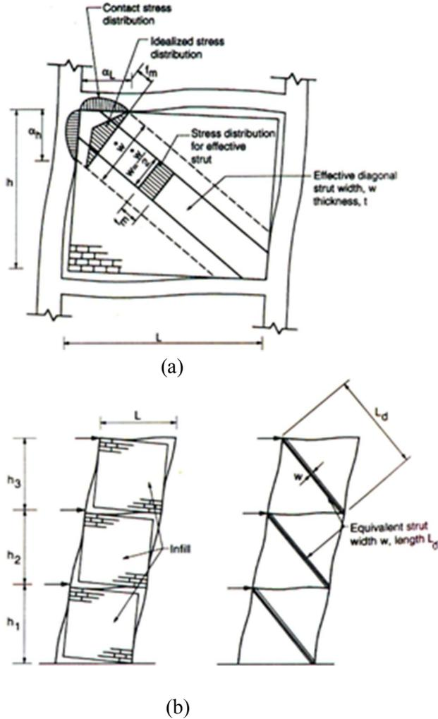
Figure 4. (a) Equivalent diagonal strut, (b) Equivalent diagonal strut method
