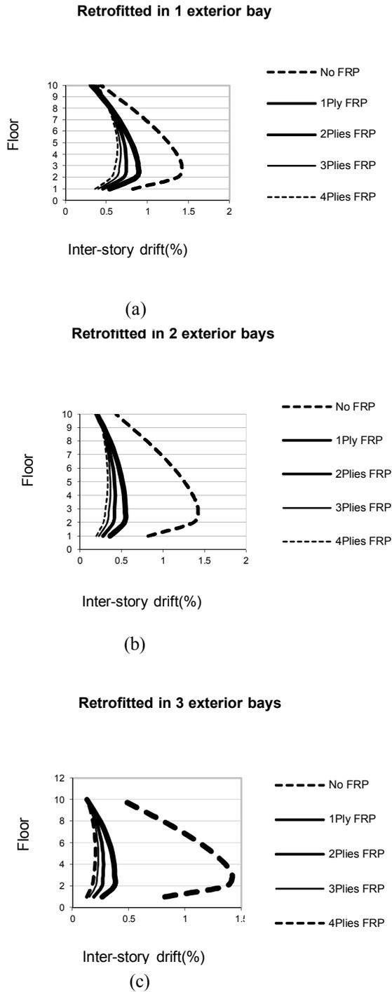
Figure 14- Comparison of inter-story drifts with different bays and plies
