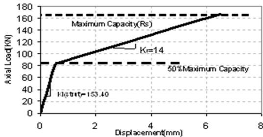
Figure 7. Equivalent behavior of strut element
