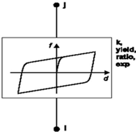
Figure 5. Nonlinear behavior of Nlink element (Plastic1)
