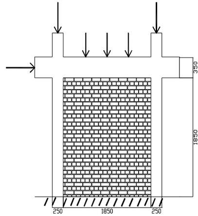
Figure 1. Applied loads in each specimen
