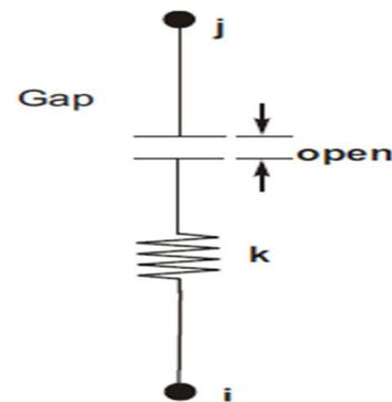
Fig 2. Gap element in SAP2000 (In this study open=0)
