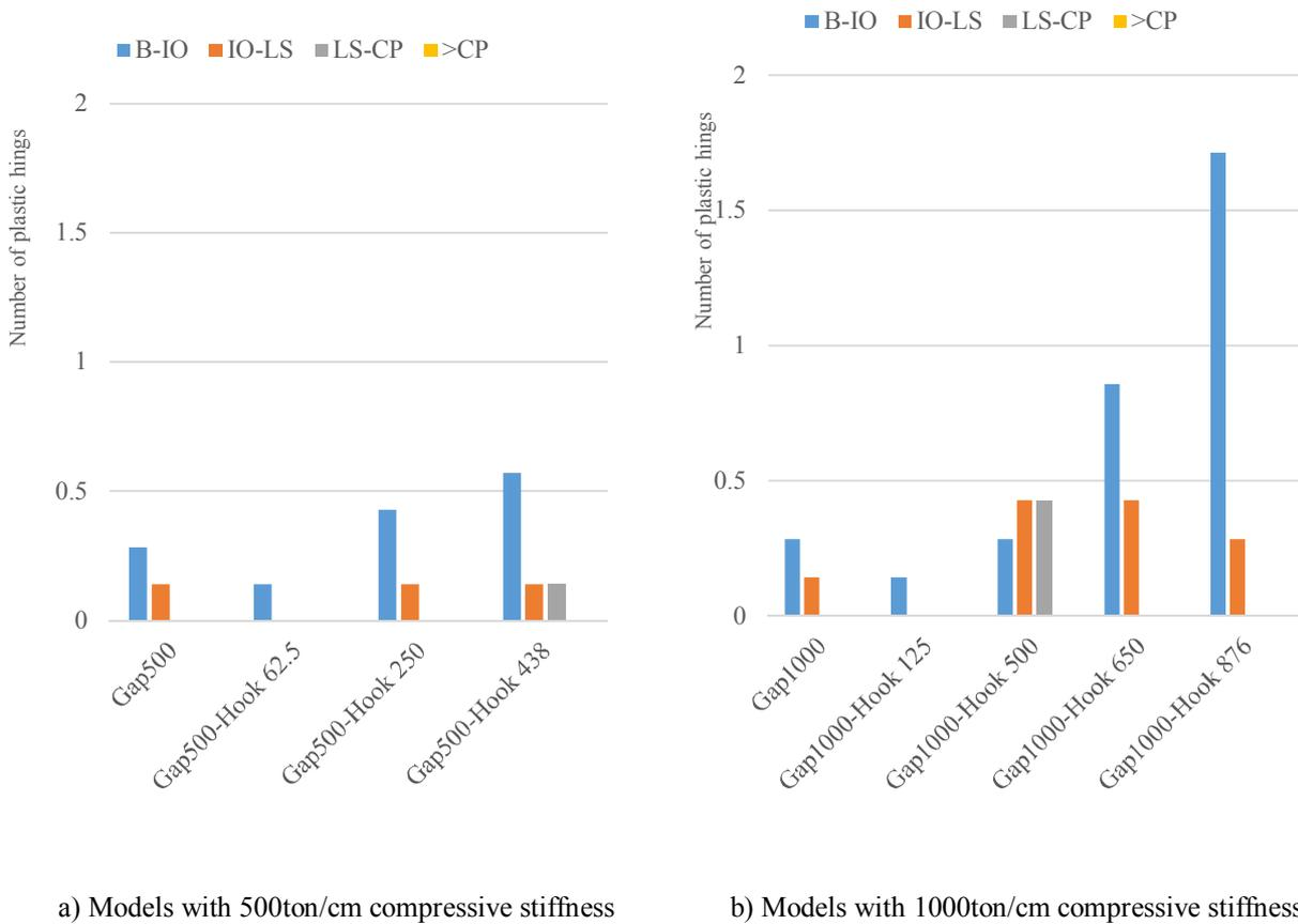
Fig. 9 Comparison of models performance level in 0.7g intensity level
