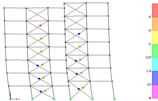
Fig. 11. Location of plastic hinges for seven-storey building with 1.2 split level in CBF system
