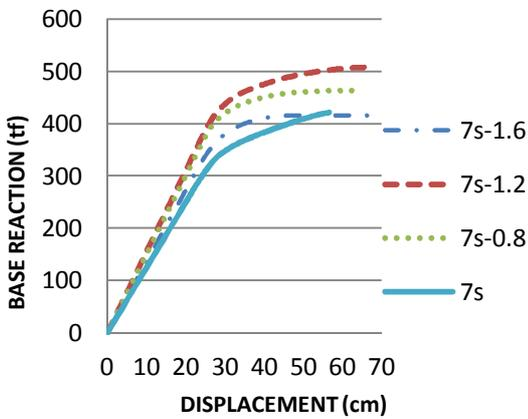
Fig. 7. Capacity Curve of moment frames for normal and duplex 7-storey buildings with different level differences
