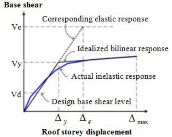
Fig. 1. Lateral load–roof displacement relationship of a structure.
