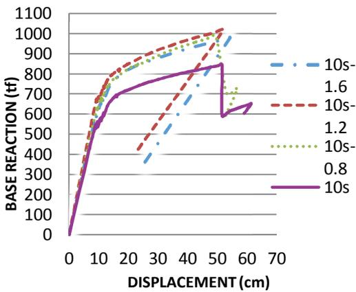
Fig. 8. Capacity Curve of braced frames for normal and duplex 10-storey buildings with different level differences
