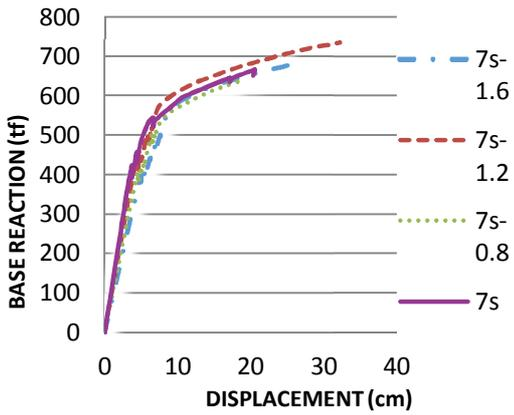
Fig. 6. Capacity Curve of braced frames for normal and duplex 7-storey buildings with different level differences
