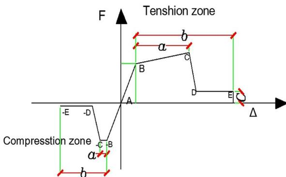
Fig. 3. Constitutive model of Bracing, beams and columns
