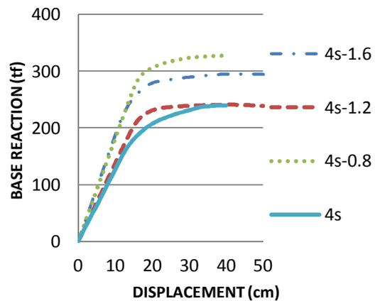
Fig. 5. Capacity Curve of moment frames for normal and duplex 4-storey buildings with different level differences
