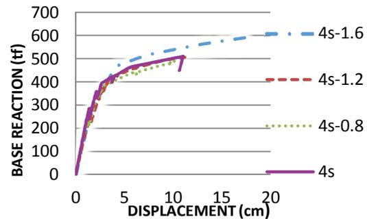
Fig. 4. Capacity Curve of braced frames for normal and duplex 4-storey buildings with different level
