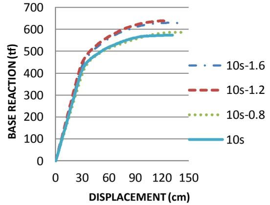
Fig. 9. Capacity Curve of moment frames for normal and duplex 10-storey buildings with different level differences
