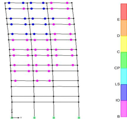
Fig. 10. Location of plastic hinges for seven-storey building with 1.2 split level in special MRF system
