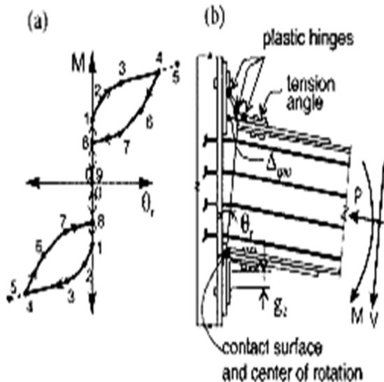
Figure 2. a) Behavior moment- rotation b) transformation of post-tensioned connection [3]
