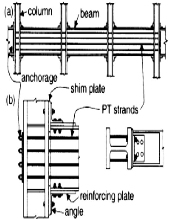
Figure 1. a) Schematic view of the steel moment frame pulled a class b) Connection Details [3]
