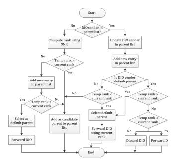
Fig.2. Flowchart to indicate forwarding rules of DIO messages to construct DAGs and compute node rank based on SNR as the new parameter to calculate ETX.
