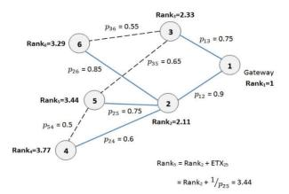
Fig.1. The procedure of the rank calculation in a DAG
