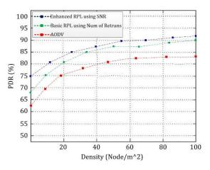
Fig. 4. Comparison of PDR performance vs. Density when using RPL with SNR, RPL with number of re-transmission, and AODV
