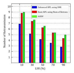
Fig. 5. Comparison of number of re-transmission vs. LSR in RPL with SNR, RPL with number of re-transmission, and AODV
