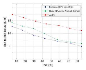
Fig. 6. Comparison of average end to end delay vs. LSR in RPL with SNR, RPL with number of re-transmission, and AODV
