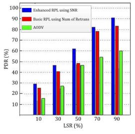
Fig. 3. Comparison of PDR performance vs. LSR in RPL with SNR, RPL with number of re-transmission, and AODV
