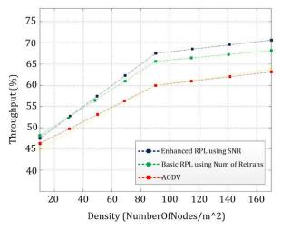
Fig. 7. Comparison of throughput vs. density in RPL with SNR, RPL with number of re-transmission, and AODV
