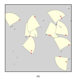
Fig. 4. A scenario of cameras and targets deployment (a) Max FoV based on target's location (b) Activated sensors in their maximal FoV.
