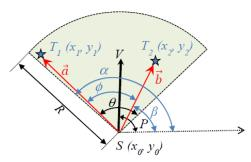
Fig. 1. FoV of a camera sensor and two targets located in.
