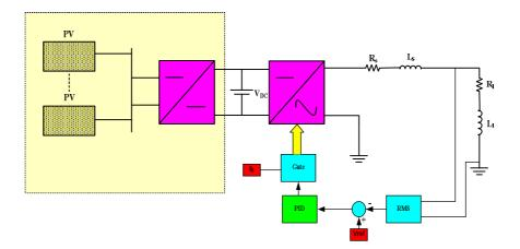
Fig.1. Photovoltaic system with battery, inverter and load
