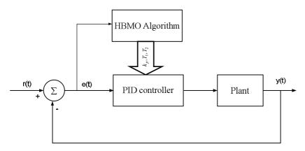
Fig. 3. Schematic of the proposed controller designing
