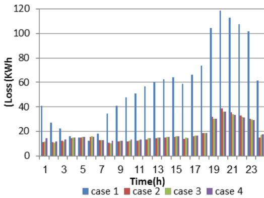
**Fig. 9.** Comparison of daily real power losses in 33-bus distribution system in four cases
