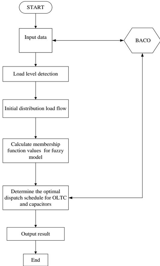
**Fig.3.** Flowchart of the Volt/VAr control algorithm
