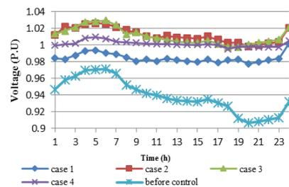
Fig.7. Voltage profile for bus-18 for different cases in 33-bus IEEE distribution system
