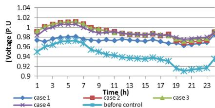
**Fig. 12.** Voltage profile for bus 65 in 69-bus distribution system for different cases
