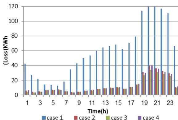
**Fig. 15.** Comparison of daily real power losses in 69-bus distribution system in four cases
