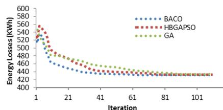
Fig.10. Convergence characteristics of the GA, HBGAPSO and BACO for the best solutions in case 3
