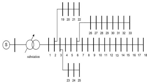
**Fig. 4.** A single line diagram of IEEE 33-bus distribution system
