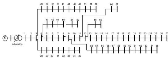
**Fig. 11.** A single line diagram of 69-bus IEEE distribution system
