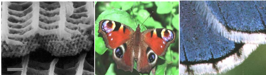
Fig.1. natural photonic crystal available at butterfly wing- Right figure indicates optic microscope from butterfly wing and left figure shows its electron microscope and periodicity of its structure [4].
