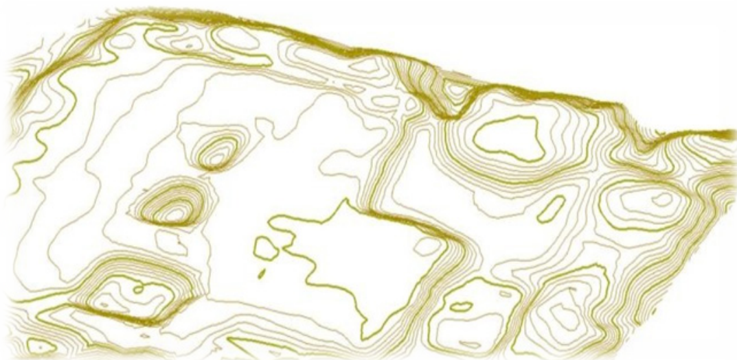
Fig. 6: Rate curve resulting from dense point cloud processing of Apadana Palace area of Susa
