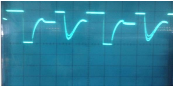
Fig.9: Output Voltage Wave Form Across Diode
