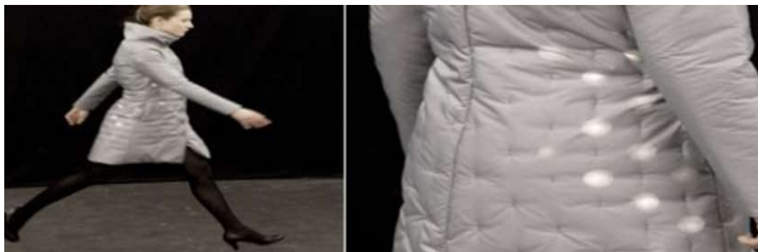
Figure 12: LED Jacket with an embedded accelerometer
