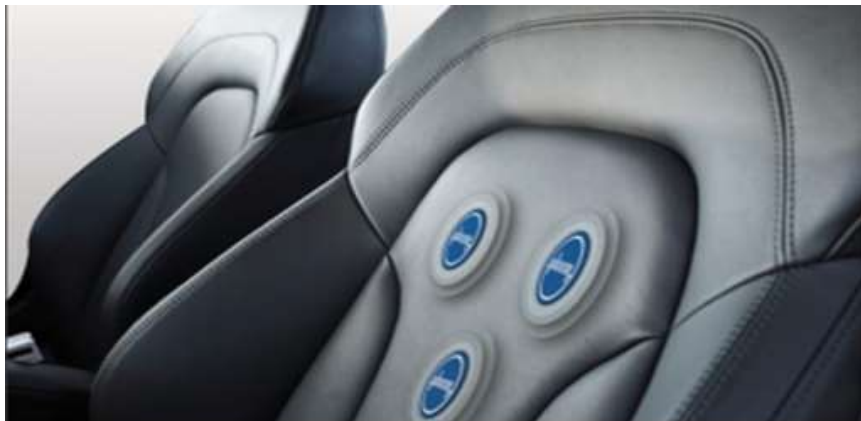
Figure 19. Car cover fitted with advanced wave-guiding technology to form a wearable antenna.
