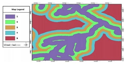
Fig. 8 - Classifying and reassigning scores to the layer of distance from the rivers
