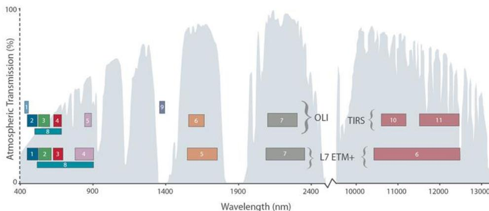
**Figure 4.** Wavelengths received in Landsat 7 and Landsat 8
