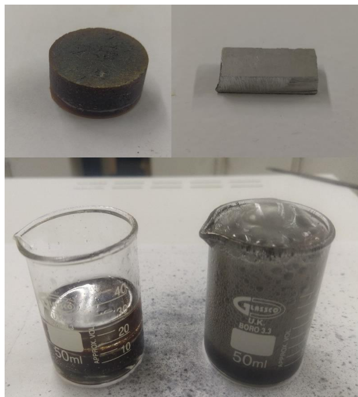
Fig.11. Image of corrosion test against acid
