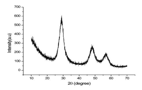
Fig. 1. XRD pattern of ZnS nanoparticles synthesized by aqueous chemical method
