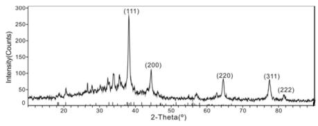
Fig 2. XRD pattern of the TiO<sub>2</sub> nanoparticles
