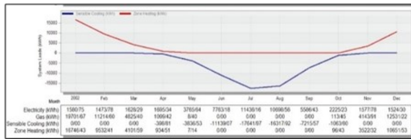
Figure 10. The graph of heating and cooling energy consumption in the sample building regarding the canopy with a protrusion of 0.5 meters in the graphic form
