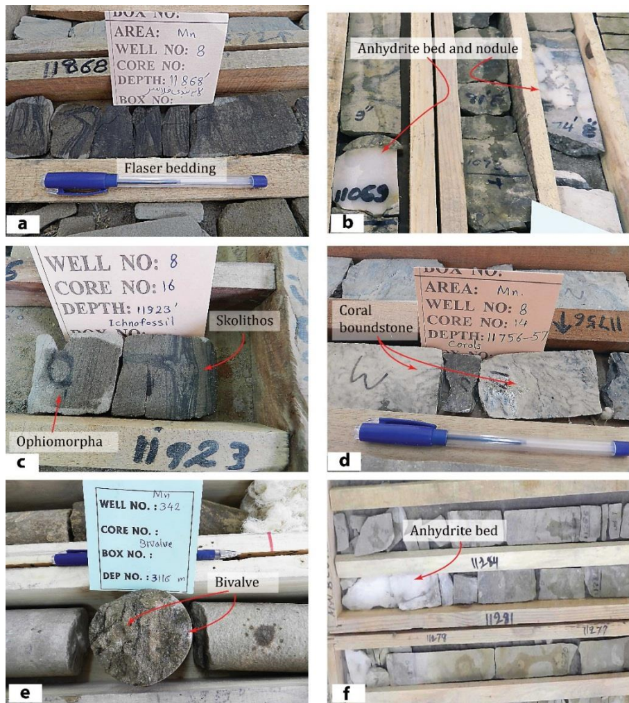
Fig 10. Sedimentary characteristics of the Asmari Formation. a. Flaser bedding, Well 8, depth of 11868'; b. Anhydrite nodules, Well 8, depth of 11069-11075'; c. Trace fossils (Ophiomorpha), Well 8, Core d = 5 cm; d. Coral boundstone, Well 8, depth of 11756'; e. Bivalves, well 342, depth of 3116 m; f. Anhydrite interval, Well 8, depth of 11281-11282'.
