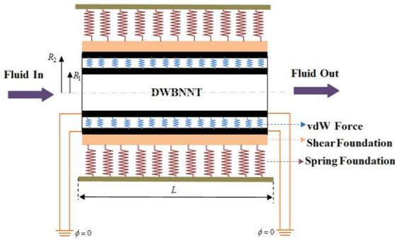
**Fig.1** A DWBNNTs conveying viscous fluid embedded in an elastic medium modeled as the nonlocal Timoshenko nanobeam.
