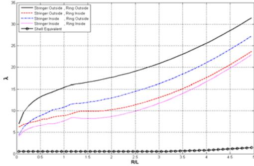
**Fig. 9** Axial pressure buckling parameter  $\lambda$ , for stringers and rings stiffened cylindrical shell ( $R/L < 5$ ).
