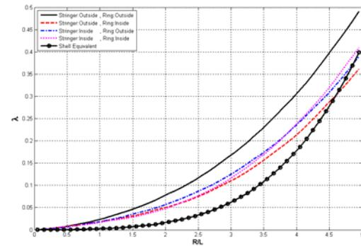
**Fig. 11** Lateral pressure buckling parameter  $\lambda$ , for stringers and rings stiffened cylindrical shell ( $R/L < 5$ ).
