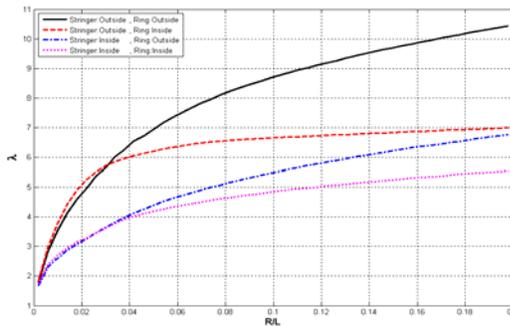
**Fig. 10** Axial pressure buckling parameter  $\lambda$ , for stringers and rings stiffened cylindrical shell ( $R/L < 0.2$ ).
