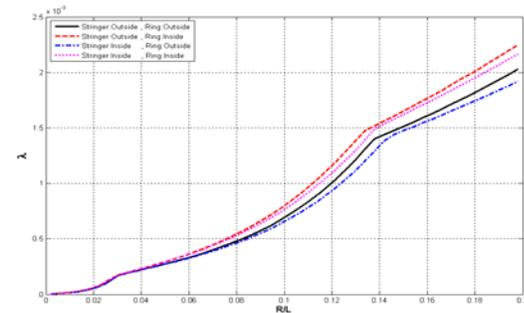
**Fig. 12** Lateral pressure buckling parameter  $\lambda$ , for stringers and rings stiffened cylindrical shell ( $R/L < 0.2$ ).
