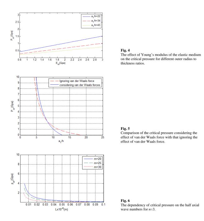
Fig. 6 shows the variation of the critical buckling load  $p_{cr}$  with respect to the tube length (*L*) for various axial half wave numbers 20, 25 and 30 (*n*=3). As can be seen from this figure that the critical buckling load decreases with increasing of the length of the nanotube for a constant radius of the outer tube ( $a_1$ ). It is also observed that the critical pressure descend very quickly with increasing the half axial wave numbers.
