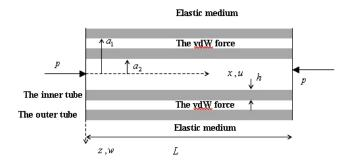
**Fig. 1** A double-walled carbon nanotube embedded in an elastic medium.
