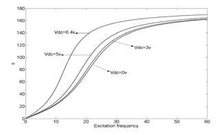
**Fig. 6** Effects of DC voltage on the phase diagram.
