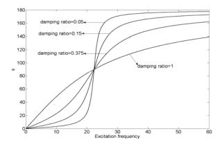
**Fig. 5** Phase Diagram for Various Damping Ratios.
