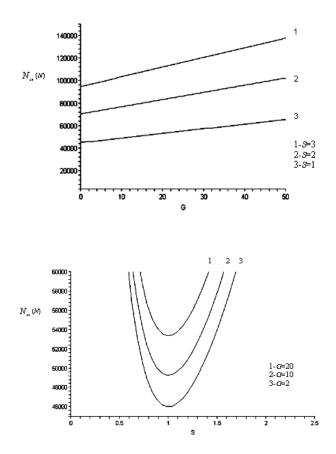
Fig. 3 Variation of buckling load vs. feedback gain for different values of S=a/b for PZT-4 (R=1).
