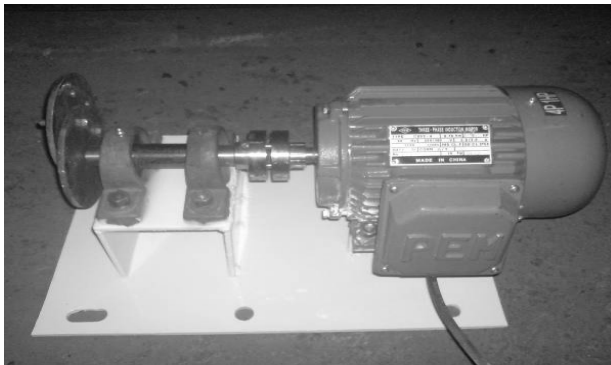
Fig.1 Vibration generating equipment.
