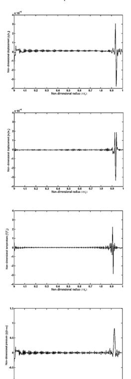
Fig. 5 Non-dimensional displacement distribution due to input  $T(1,z,t) = 10^{-3}T_0\delta(t)\sin(z)$  at non-dimensional time  $\hat{t} = 0.1$ .
