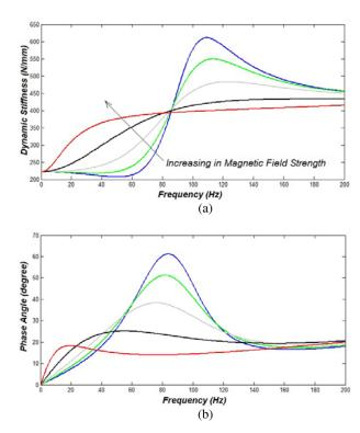
Fig. 5 Variation of the dynamic characteristics of the first design of MR mount with applied magnetic field strength; (a): dynamic stiffness and (b): phase angle.
