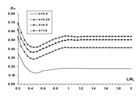
Fig. 4 Influence of  $L/R_1$  on ratio  $\rho_{cr}$  for SS<sub>3</sub> ( $\alpha = 30^\circ$ ,  $R_1/h = 100$ ,  $\upsilon = 0.3$ ).
