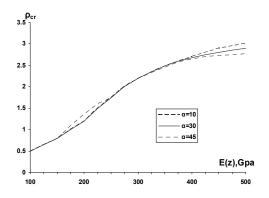
Fig. 5 Influence of E(z) on ratio  $\rho_{cr}$  for SS<sub>3</sub>  $(L/R_1 = 10, R_1/h = 100, \nu = 0.3)$ .
