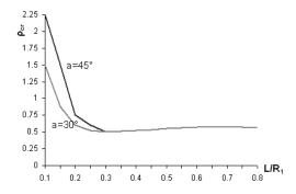
**Fig. 2** Influence of  $L/R_1$  on ratio  $\rho_{cr}$  for SS<sub>3</sub>.
