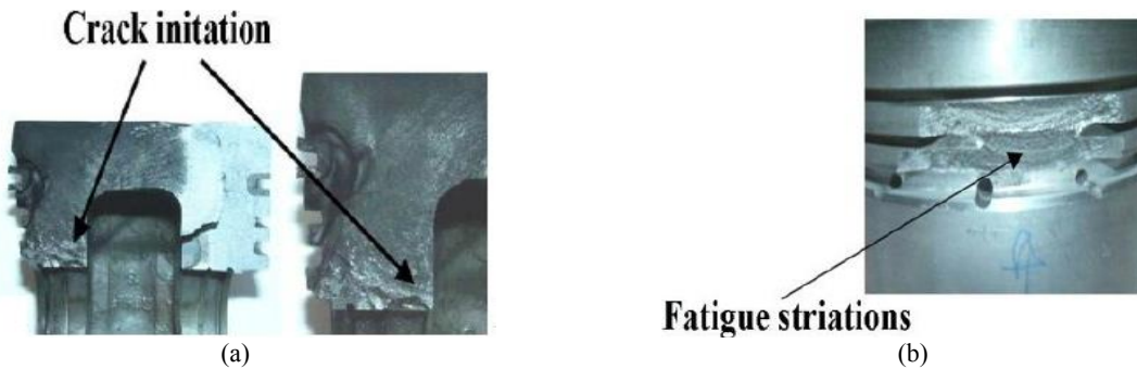
Fig.9 A damaged engine piston (a) in upper portion of piston pin and (b) on piston compression grooves [23].
