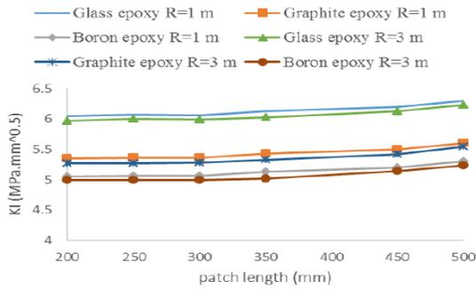
**Fig.11** The average SIF in terms of the patch length for glass, boron, and graphite-epoxy patches.
