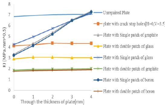
**Fig.12** SIF along the thickness of the Plate, for different repair methods.
