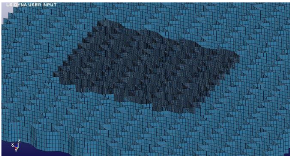
Fig.8 The finite element model of the honeycomb panel.
