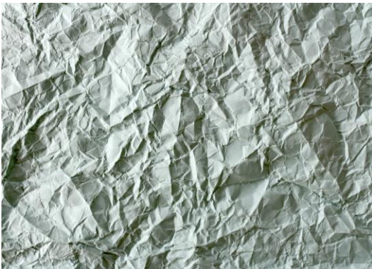
Fig.1 Crumpled paper will be much easier to stretch than when it is plane i.e. low elastic modulus.
