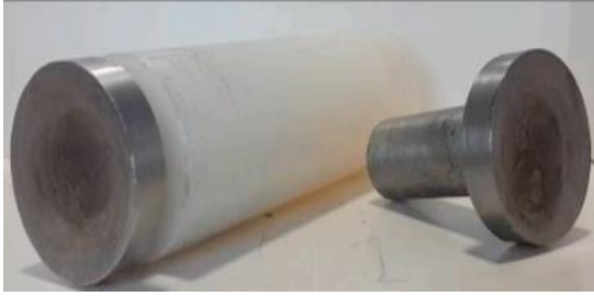
Fig.5 The striking mass in the dynamic experimental apparatus.
