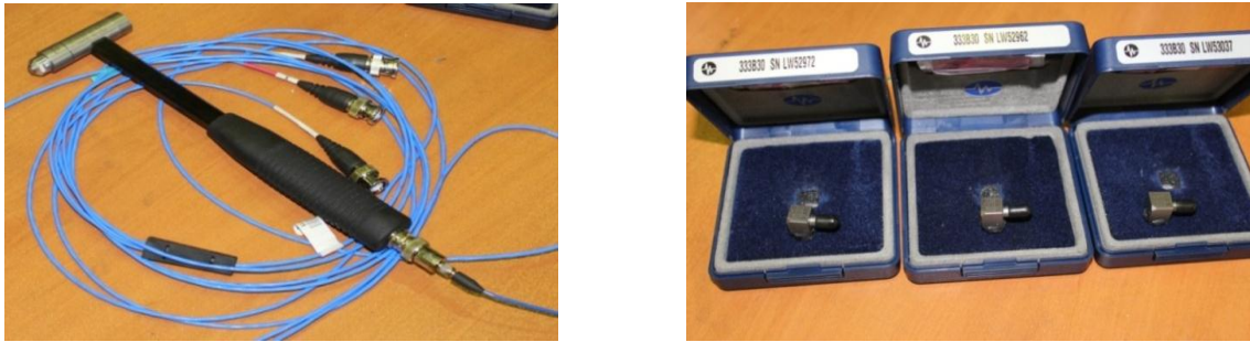
Fig.5 The PCB 086C40 hammer & the PCB 352B10 piezoelectric accelerometer.
