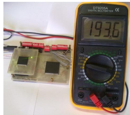
Fig. 13. FPGA test kit board.
