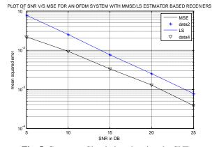
**Fig. 5.** Computer Simulation showing the SNR performances of the MMSE and LS Channel Estimation Methods on the receiver in a 64-carrier OFDM system.
