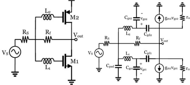
Fig. 3.(a) Resistive shunt feedback LNA with inductive series (b) its equivalent circuit model
