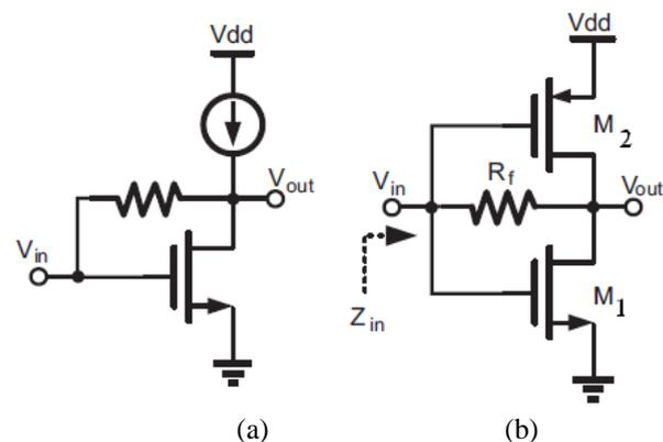
**Fig.1.** (a) Resistive-Feedback LNA.(b)With a current source
