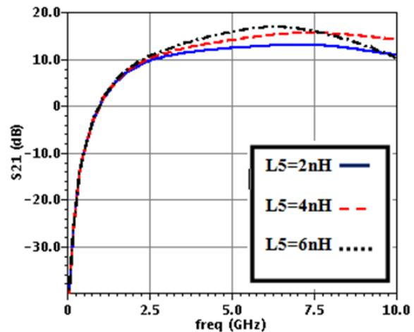
Fig. 4. Effect L<sub>5</sub> on the S<sub>21</sub>
